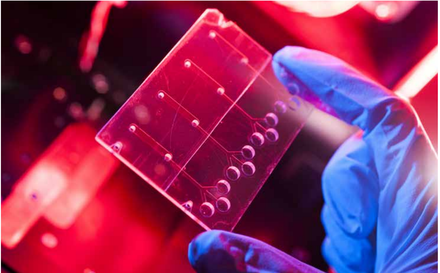
The CYBERNOSE technology breaks with traditional electronic nose design in using microfluidic channels that allow the sensors to flow continuously, eliminating the problem of sensor drift. Image: Carl Davies, CSIRO.
